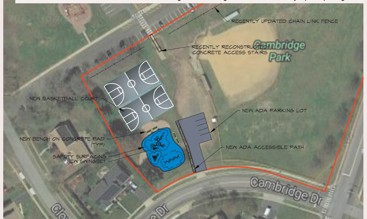
Cambridge Park site plan from project engineer T&M shows planned additions of a second basketball court, play area enhancements, new ADA-compliant parking area and path, and recently completed access stairs and chain link fence. Work is being funded through a Monmouth County Open Space grant.
